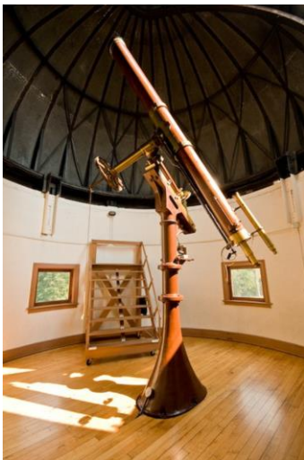
(Weighing 2,500 pounds, the 11" Merz und Mahler telescope was built in Bavaria and shipped to Cincinnati by 1845. It was manufactured during a time without power tools. Every single nut and bolt fits in a specific and non-interchangeable location on the telescope.)
